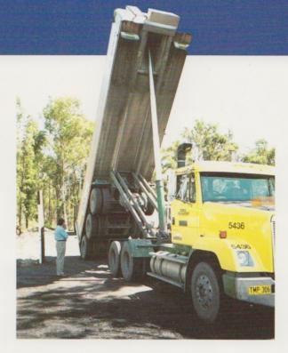
This streamlined method of construction also provides the maximum diameter at the top of the extended tube, a critical point in any tipping cylinder design. Close tube tolerances ensure the maximum power/weight ratio for most effective lift capability. A gland nut on the base tube provides easy assembly, and the one piece construction eliminates waste during manufacture.
